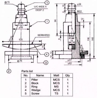
Figure 1: Lathe Single Tool post
